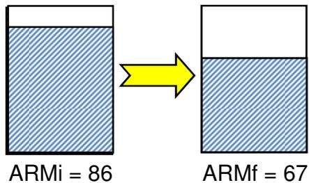
$$\begin{aligned} (P-ETP) &= -25 \text{ mm} \\ NAc &= -15 + (-25) = -40 \\ ARMf &= 100 * e^{-40/100} = 67 \\ ALT &= 67 - 86 = -19 \\ ETR &= 0 + |-19| = 19 \text{ mm} \\ DEF &= 25 - 19 = 6 \text{ mm} \\ EXC &= 0 \end{aligned}$$
