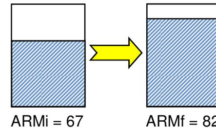
$$\begin{aligned} (P-ETP) &= +15 \text{ mm} \\ ARMf &= 67 + 15 = 82 \\ NAc &= 100 \text{ Ln } 82/100 = -20 \\ ALT &= 82 - 67 = +15 \\ ETR &= ETP = 25 \text{ mm} \\ DEF &= 0 \\ EXC &= 15 - 15 = 0 \end{aligned}$$
